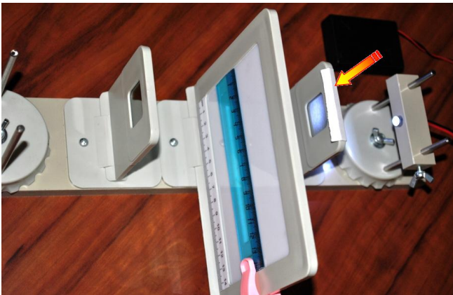
Fig. 1B Setup for the observation of birefringence in the ruler
