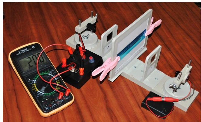
Fig. 4B Setup for measuring the transmittance of light through plastic ruler
