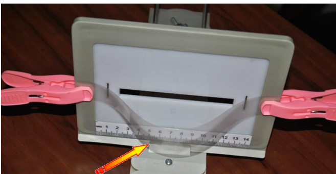
Fig. 1B Setup for the observation of birefringence in the ruler
