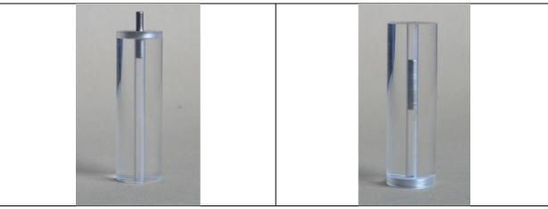
Figure 3. Photo of two magnets and a transparent hollow cylinder; the rod-magnet moves through the cylinder's hole.
