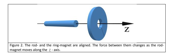
To ensure motion of the rod-magnet along the axis of symmetry (z - axis), the ring-magnet is firmly embedded in a transparent cylinder, which has a narrow hole drilled along the z - axis. The rodmagnet is thus constrained to move along the z - axis through the hole (see Fig. 3). The magnetization of the magnets is along the z - axis. The hole ensures radial stability of the magnets.
