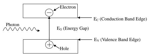
Fig. II-1 Schematic diagram of an electron-hole pair generated by a single photon in a semiconductor.
