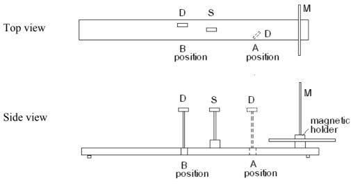
Fig. 2.1. Study of the wave interference. Position A: The detector is placed between Source and Mirror. Position B: The detector is placed behind the Source. S- Source, M-Mirror, D-Detector
