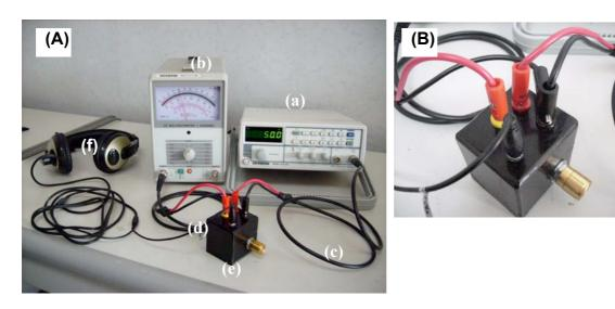
Figure 4.1 (A). Connections of the apparatuses. (B) Connections of the leads to the rheostat: plug in the red lead from the function generator to the red socket and black lead to the black socket; connect the red lead of AC millivoltmeter to yellow socket and the black lead to the black socket; and plug in headphone lead to the headphone socket.
