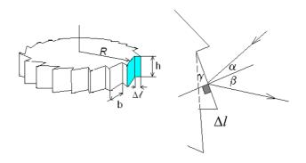
Figure 1. The saw tooth of the rotating disk
