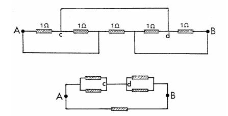
The equivalent drawing of the circuit shows that the resistance between point c and point A is  $0.5\Omega$ , and the same between point d and point B. The resistance between points A and B thus consists of two connections in parallel: the direct  $1\Omega$  connection and a connection consisting of two  $0.5\Omega$  resistances in series, in other words two parallel  $1\Omega$  connections. This yields
