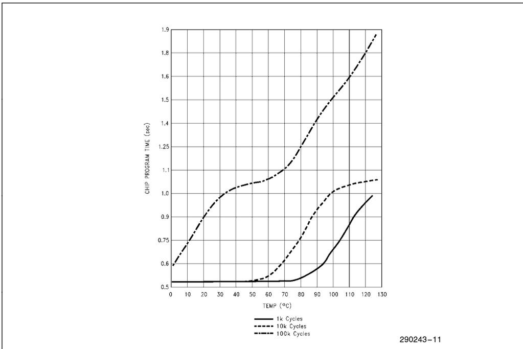
Figure 8. 28F256A Typical Program Time at 12V
