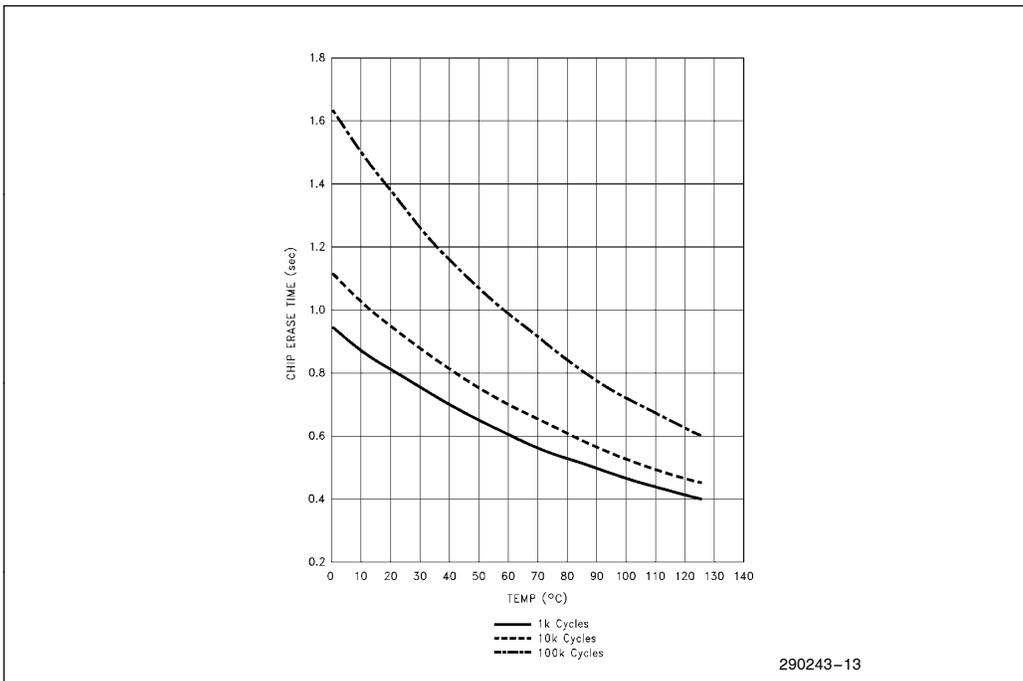
Figure 10. 28F256A Typical Erase Time at 12.0V
